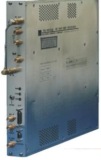
The WJ-8635 is a fully synthesized, general-purpose HF/VHF/UHF receiver tunable from 20 to  $1000\,\mathrm{MHz}$ , and extendable down to  $0.5\,\mathrm{MHz}$  or up to  $2.4\,\mathrm{GHz}$ .
